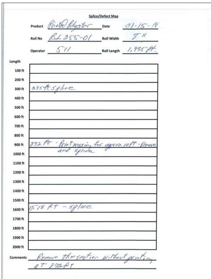
**FIGURE 1.** Splice/defect map from the customer should include details such as the length where the splice is on each and every roll, and where and how it is marked or flagged.
